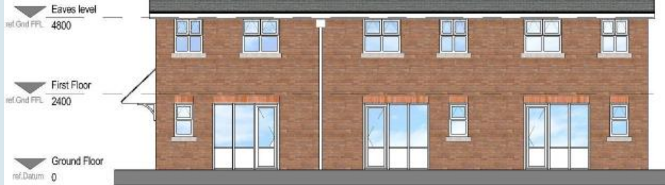
Rear Elevation - Facing North Boundary
